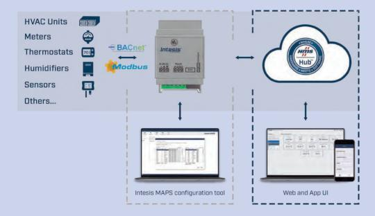
Intesis ST Cloud Control is a cloud based solution from HMS which enables easy monitoring and control of any BACnet or Modbus device from an end user oriented app and a web based dashboard.
